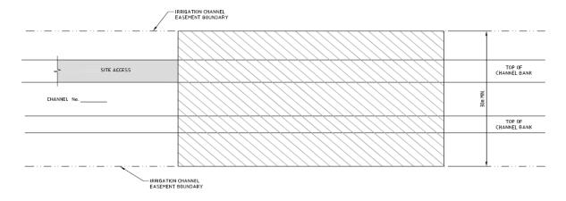
Figure 4 - Typical channel lining site footprint
