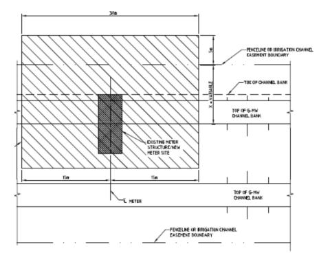
Figure 2 - Typical meter site footprint
